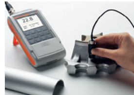
ISOSCOPE® FMP30 using probe FTA3.3H
