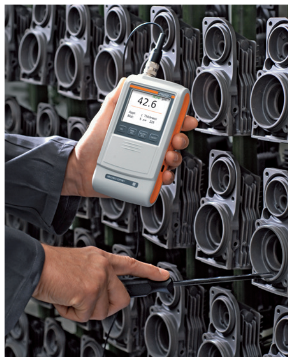
Measurements using the internal probe FAI 3.3-150
